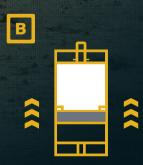
The hydraulic system is pressurized. The system pressure exceeds the precharge pressure, and the fluid flows into the accumulator.
